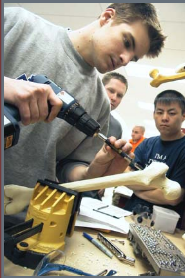
M.E. Bioengineering students practice the surgical repair of a hip fracture in Kettering's Fracture Lab.
